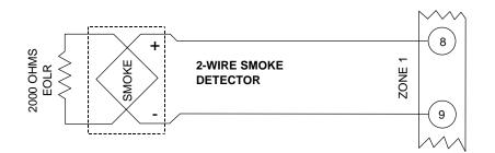
Figure 8. 2-Wire Smoke Detector Connected to Zone 1
